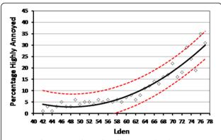
**Figure 4 The %HA with road traffic noise.** The data points are the %HA within each 1 dB interval of exposure over the  $L_{\rm den}$  range of 42 to 77 dB. The best fit quadratic exposure-response regression model is shown, together with 95% upper and lower confidence bounds.
