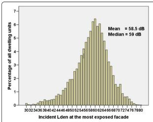
Figure 3 Distribution of the exposure to road traffic noise of all dwelling units in the sample (n = 10,077). These are predicted by 3D noise mapping. The estimates are of  $L_{den}$  in 1 dB bins for levels above 30 dB.
