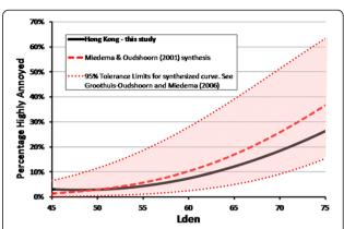
Figure 8 Comparison of the exposure-response model of %HA with road traffic noise in Hong Kong with that synthesized by Miedema and Oudshoorn [18]. The 95% tolerance interval of the synthesized exposure-response curve from the meta-analysis of 26 previous studies [18] is shown shaded.
