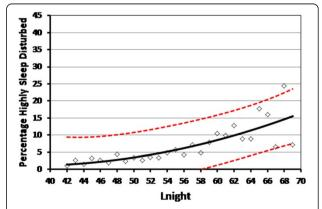
**Figure 5 The %HSD by road traffic noise.** The data points are the %HSD within each 1 dB interval of exposure over the  $L_{\text{night}}$  range of 42 to 69 dB. The best fit quadratic exposure-response regression model is shown, together with 95% upper and lower confidence bounds.
