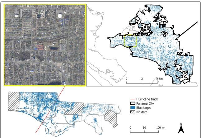
**Fig. 1** The aerial image (top left) shows an urban area with a number of roofs covered by blue tarps. \*The image covers one square mile in Panama City, FL (top right). The blue tarps in the study area are more densely distributed near the hurricane track but were detected throughout much of the study area (bottom)
