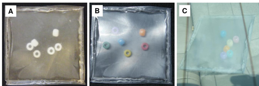
Figure 7 UV-detecting beads change color when sunlight passes through Tritan™ TX2001 plaques. Demonstration that sunlight can pass through a sealed pouch formed from Tritan™ TX2001 to cause the UV-detecting beads to change color. A. Unexposed beads in Tritan pouch. B. Beads in Tritan pouch exposed to natural sunlight. C. Beads in Tritan pouch exposed to natural sunlight through a window. A color change in the beads shows that UV radiation has been captured by a bead. The change to one color versus another color has no significance.
